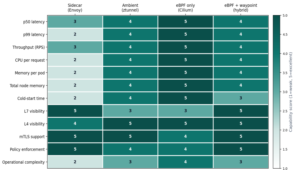
Figure 7. Capability scorecard across twelve operational dimensions for the three data-plane patterns and the hybrid eBPF-plus-waypoint configuration.
